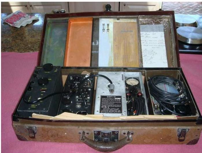
This unit was similar to other suitcase spy radio sets developed by various European countries during WW2. Its crystal controlled transmitter provided a CW output of about 8-15 watts.
